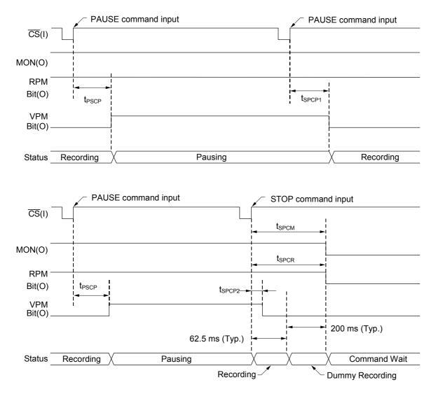
(NOTE) If the STOP command is input while recording is suspended by the PAUSE command, the LSI resumes recording and keeps on recording until the last address of the current page is reached. This "lag" recording time is about 62.5 ms (Typ.).
