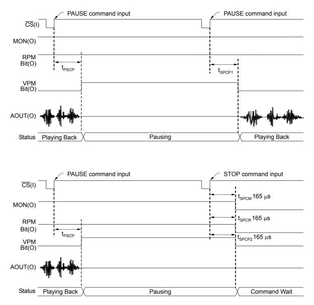
The following charts show timings for pausing playback by using the PAUSE command at 6.4 kHz sampling frequency.
