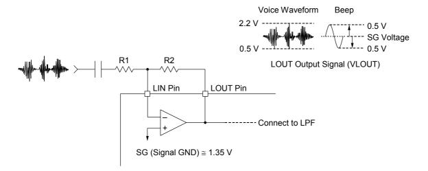
The LSI has a built-in OP amplifier to amplify incoming analog source signal. The inverting input pin to the OP amplifier (LIN pin) and the output pin from the OP amplifier (LOUT pin) are available. The non-inverting input is internally connected to the Reference Voltage (Signal Ground 1.35 V).
