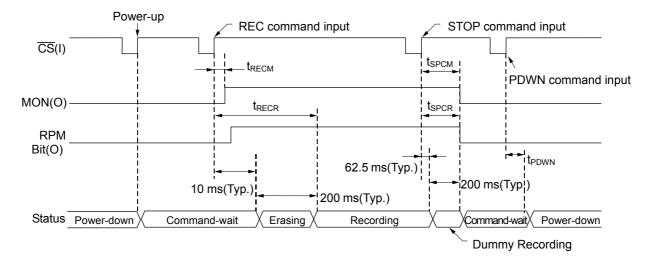
(Note 1) It takes about 210 ms (Typ.) for the LSI to start actual recording after the REC command input, as the LSI first erase 1 sector before it can start recording.
