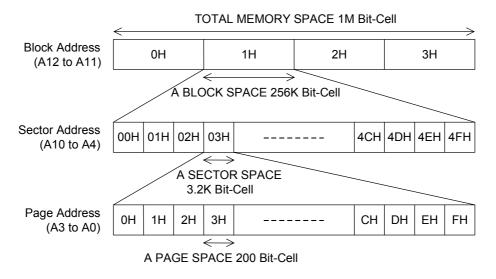
Address Assignment to Define Block, Sector and Page Address for Start and Stop Address
